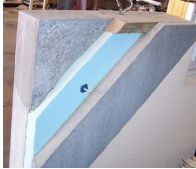
Figure 4: Cut-away View of High Mass Wall Panel (With 2 Inches of Extruded Polystyrene)
