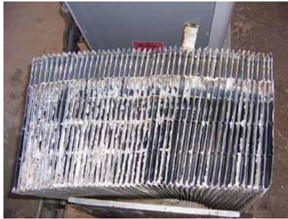
Figure 23: Evaporative Cooler Indirect Media After Two Cooling Seasons
