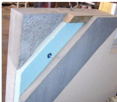
Figure 4: Cut-away View of T-Mass Wall Panel (With 2 Inches of Extruded Polystyrene)
